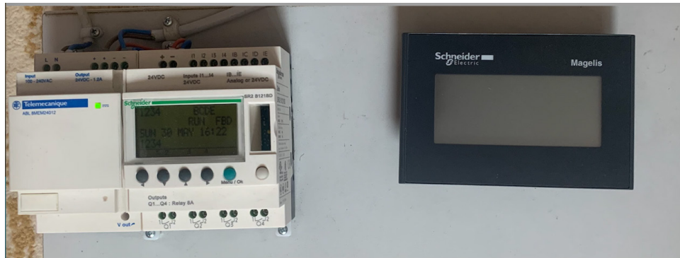
Fig. 9. Smart relay Zelio SR2 B121BD & HMI Magelis [2].
