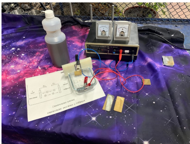
Fig. 7. Galvanizing` by electrolysis.
