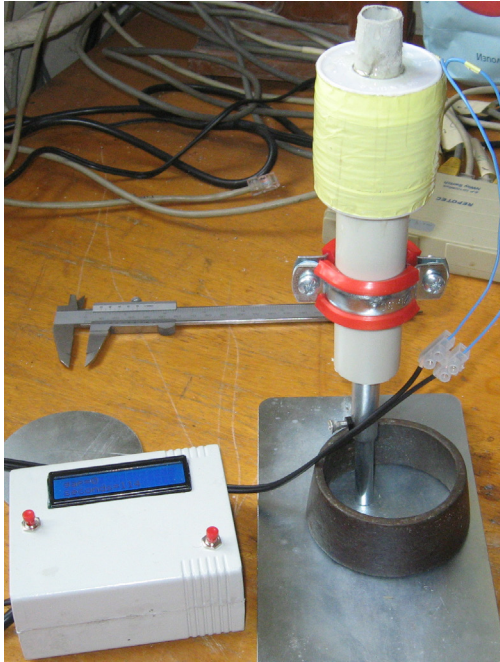
Fig. 1. Device to measure the hardening of cement mixtures.
