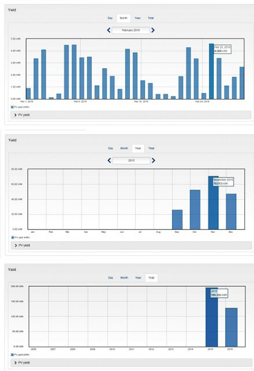
Fig. 3. Displays of PV yield monitoring by days, months and years.
