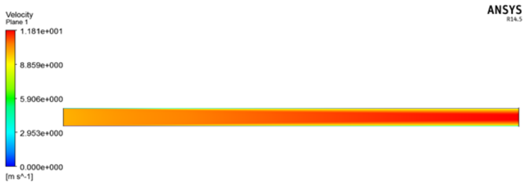
Fig. 3B. Velocity field in a longitudinal cross section at turbulent flow.
