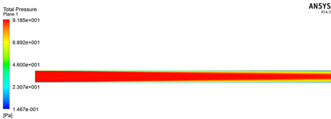
Fig. 3C. Total pressure (relative) in a longitudinal cross section at turbulent flow.
