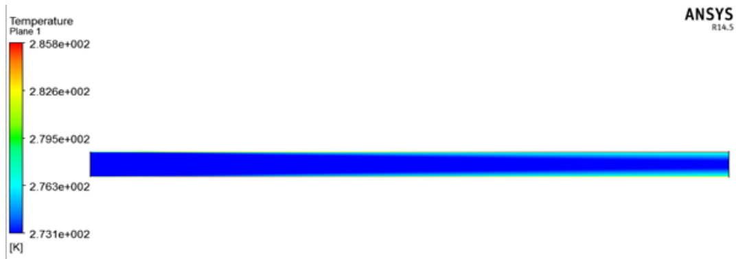
Fig. 3A. Temperature field in a longitudinal cross-section at turbulent flow.
